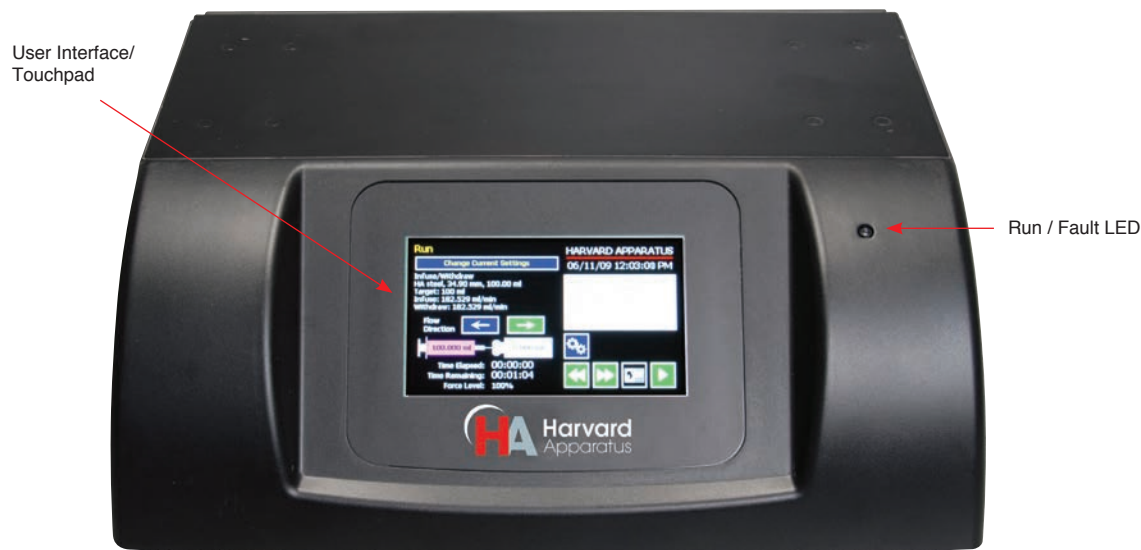
Front view of the PHD ULTRA™ Nanomite Control Box pump showing important components and controls.
